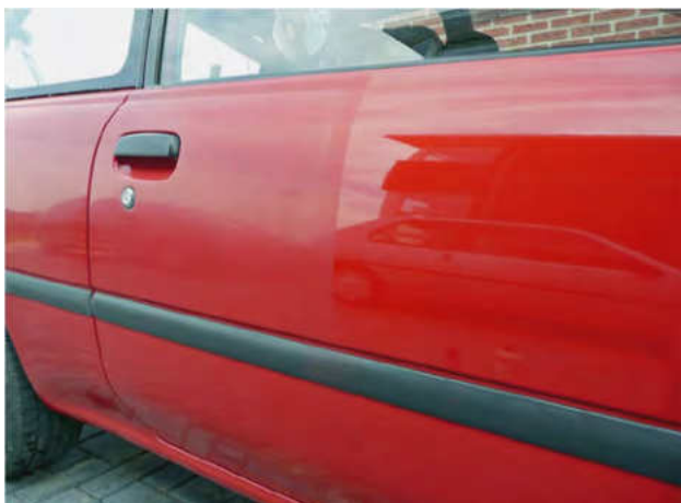
Figure 8 This image shows a variation in glossiness due to environmental factors. Photo: www.stylingspecialisten.nl .
