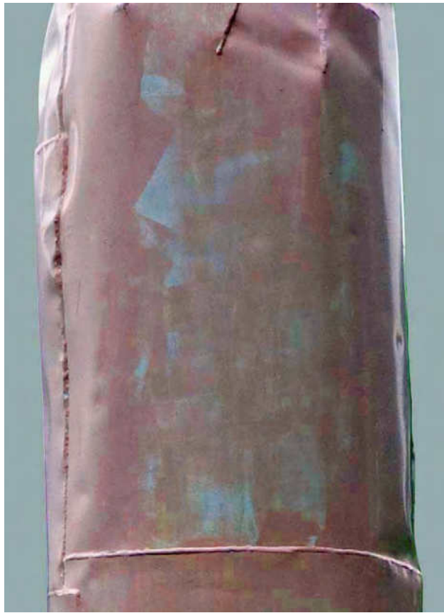
Figure 3 Detail of Flause , showing the effects of sunlight on the paint. The red in the pink color has been bleached out significantly.
