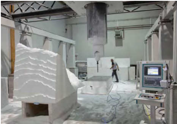
Figure 4 Rough cut of polystyrene by a 5-axis milling robot in the in-house milling center. Photo by Katalin Deér.
