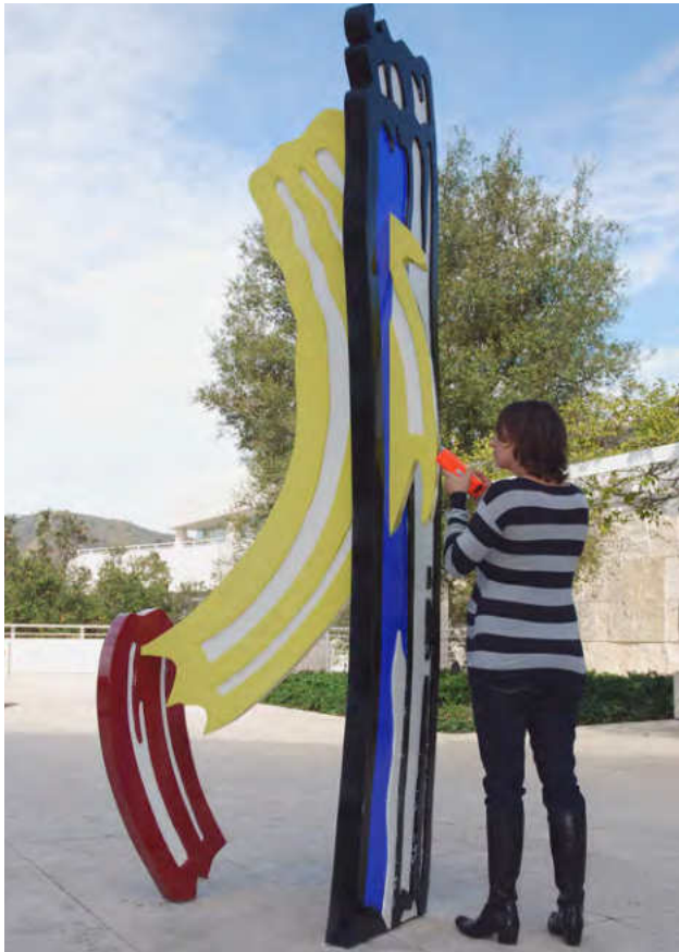
Figure 12 Rachel Rivenc takes a measurement of paint layers using a handheld FTIR instrument on Roy Lichtenstein's sculpture Three Brushstrokes . © Estate of Roy Lichtenstein.
