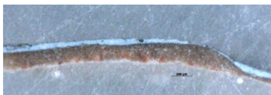
Figure 5. Cross-section viewed at 100x (OM image): Sample from blue colour on the cloak of the Virgin.
