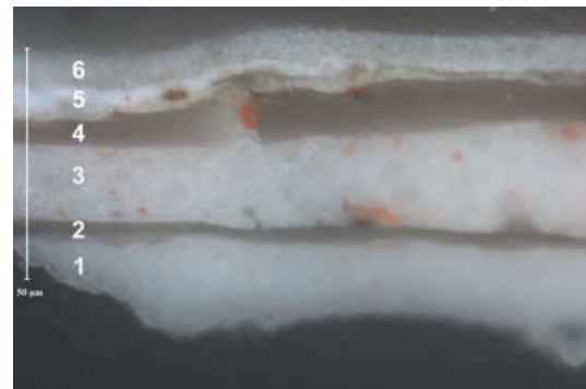
Figure 5. Cross-section sample of flesh area that shows no fluorescence under UV illumination and shows two distinct layers of titanium dioxide as anatase (Layer 5) and rutile (Layer 6). © The J. Paul Getty Museum, Los Angeles.
