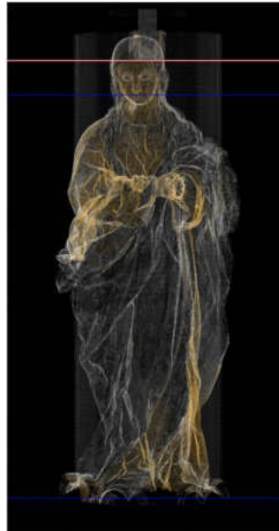
Figure 5. CT analysis. 3D transparency reconstruction showing the location of gold leaf under the upper polychromy.
