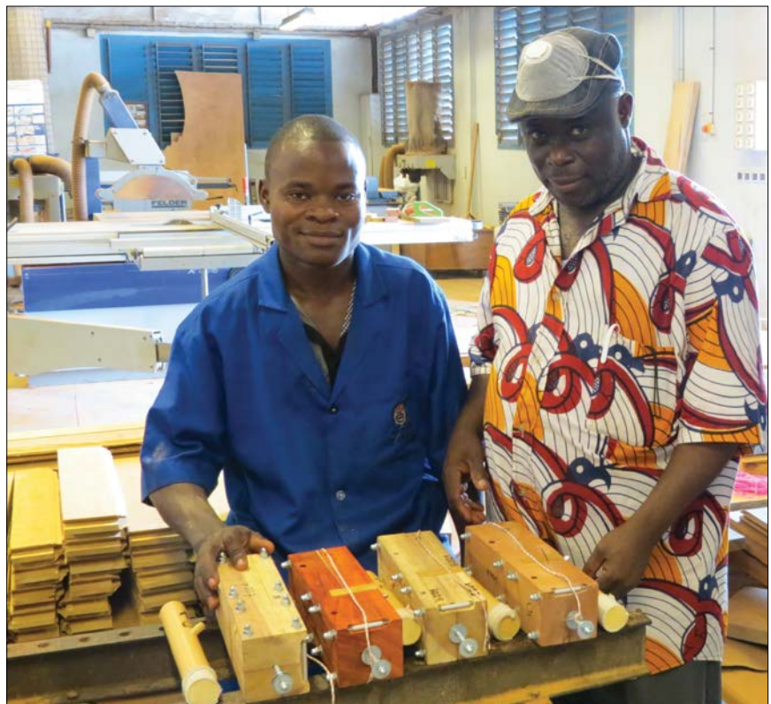
Community artisans receive training in the manufacture and use of EL@OUT,* an “ambush” version of a chilli-pepper dispenser made of wood designed to discourage elephants from damaging crops
