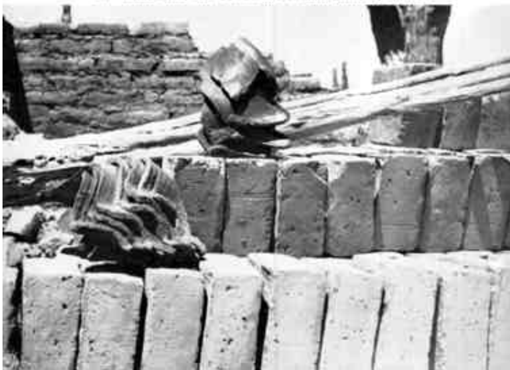
39. Adobes fired with cardón and roof tiles melted by the heat.
