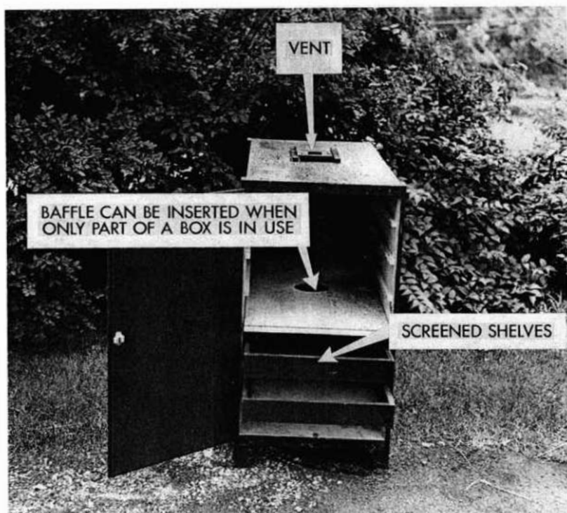
Figure 4.—Interior of an artificial drying box, showing drying racks.
