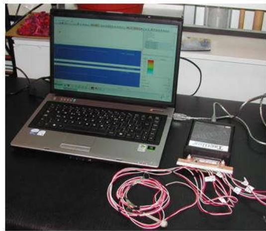
Figure 1.8: The Tactilus® Freeform Sensor System V3.1.27 (2007) shown with the hub connected via the USB cable to the Windows based software programme.
