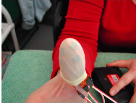
Figure 1.12: Image showing the arrangement of sensors during an experiment. The sensors were held in place by a cut-off thumb section of a latex glove.
