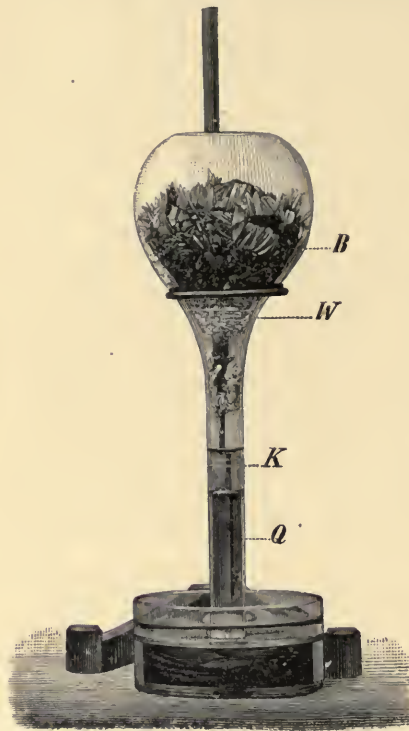
FIG. 211.—Experiment to demonstrate respiration. The inverted flask ( B ) is partially filled with flowers, which are held in place by the plug of cotton ( W ). Through the absorption of the carbonic acid exhaled in respiration, by the solution of caustic potash ( K ), the mercury ( Q ) rises in the neck of the flask.
