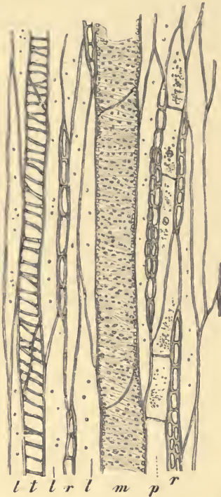
FIG. 149.—Tangential section of the wood of Tilia ulmifolia . m , Pitted vessel; t , spiral tracheides; p , wood parenchyma; l , wood fibres; r , medullary rays. ( \times 160 .)
