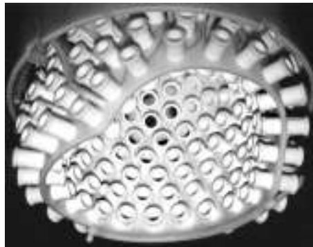
Figure 7.2. Photograph of 1st-order gradiometer sensors in the helmet area, 143 channels.
