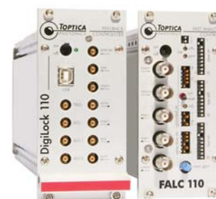
Fig. 5: DigiLock 110 and FALC 110: modules for linewidth narrowing.
