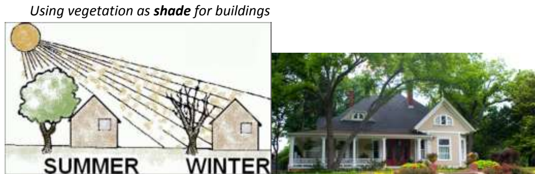
Fig. 64 (left) Strategic placement of deciduous plants will help when keeping a person cool in summer and warm in winter as trees lose their leaves (right)A house is surrounded by trees that help managing winds and sunlight
