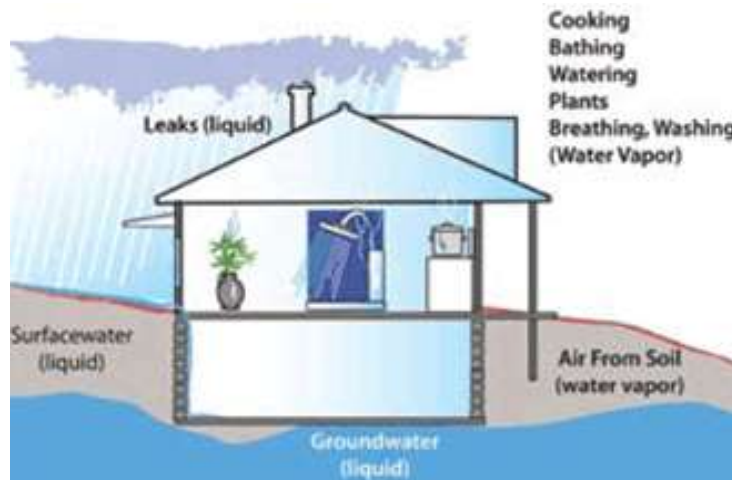
Fig. 73 Demonstration how humidity formed in building
