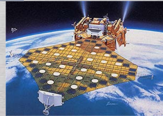
Deployable solar panels (K. Miura)
