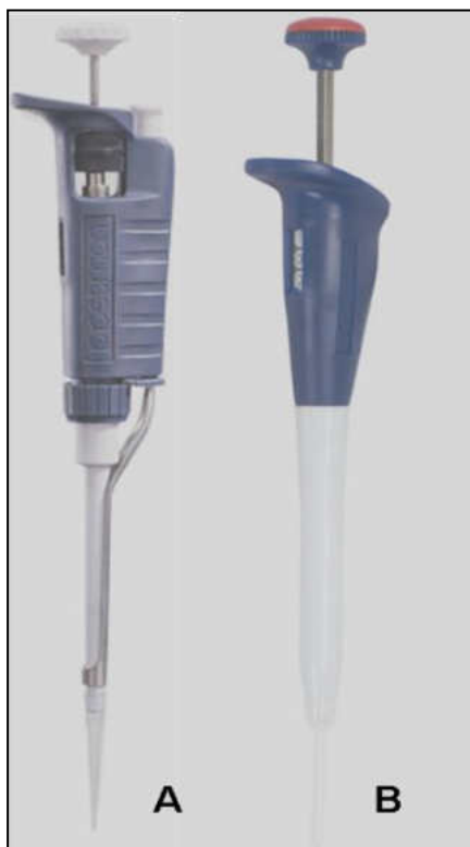
Figure 2-1. (A): Air displacement automatic pipette, (B) Positive displacement automatic pipette. (Image courtesy of Gilson UK)
