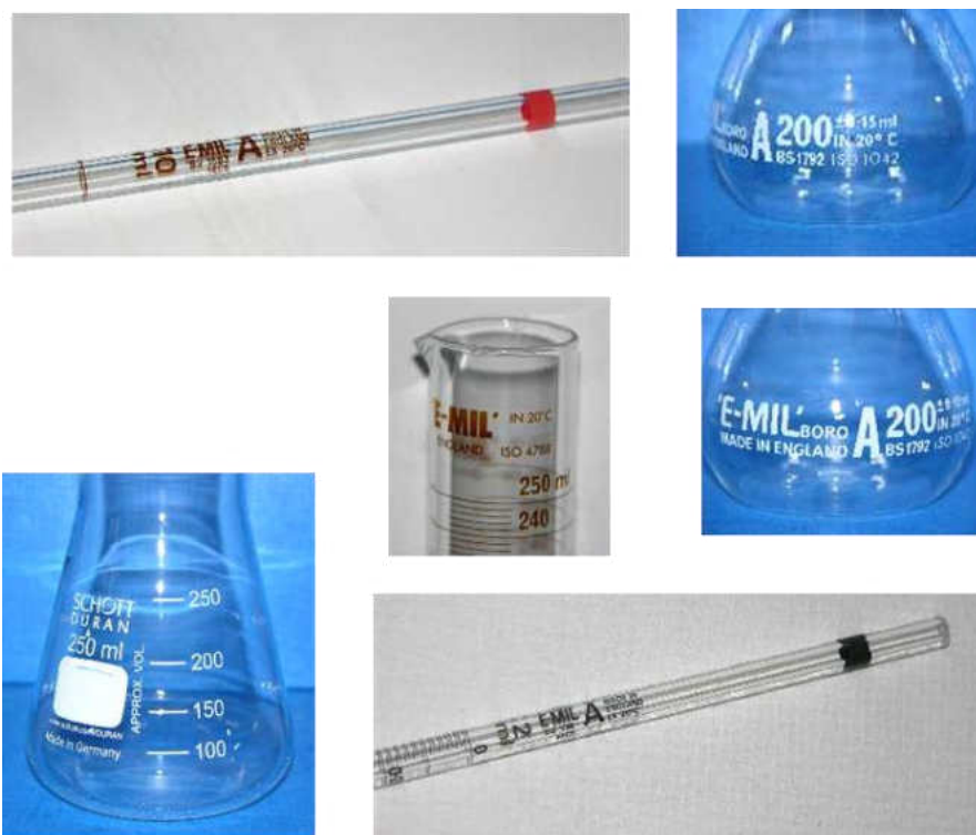
Figure 2-11. Illustrations of markings on volumetric glassware
