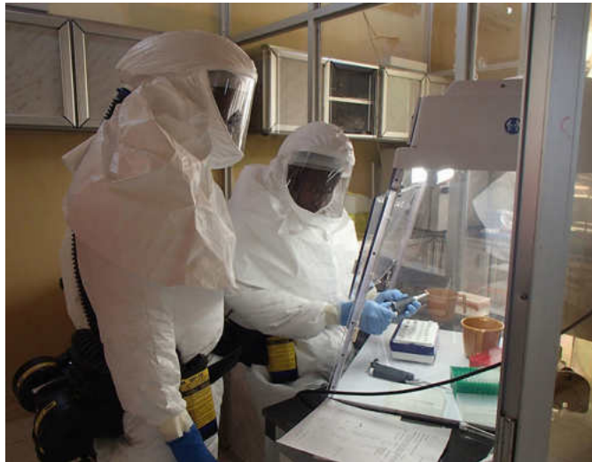
Figure 1.15 Researchers working with Ebola virus use layers of defenses against accidental infection, including protective clothing, breathing systems, and negative air-pressure cabinets for bench work. (credit: Randal J. Schoepp)
