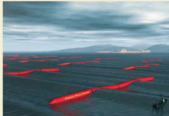
7.12 c > The Pelamis wave energy transformer floats on the ocean like a giant sea snake. It consists of several segments which move against each other and build up hydraulic pressure. This in turn drives a turbine. A new Pelamis generation is currently under construction.
