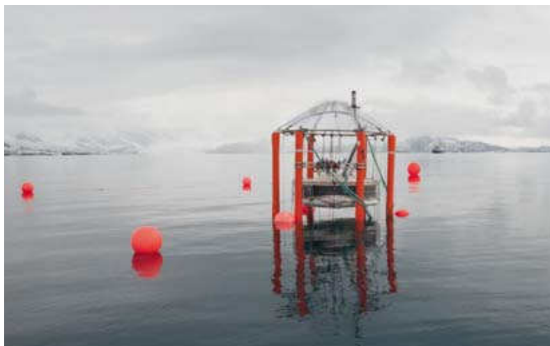
2.5 > In order to determine the effect of increasing atmospheric CO 2 concentrations on the ocean, an international research team enriched seawater with CO 2 in floating tanks off Spitsbergen, and studied the effects on organisms.
